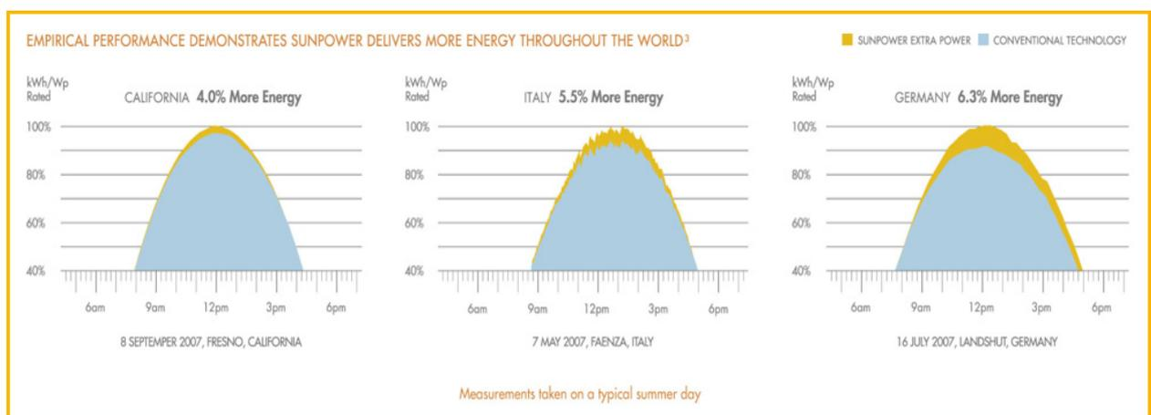
**Source:** SunPower Customers; comparisons at same site with identical inverters. System production output normalized to total solar panel factory test power.
